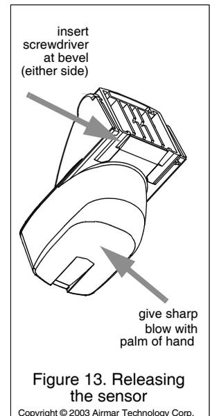
Figure 13. Releasing the sensor
