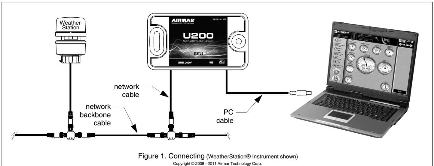
Figure 1. Connecting (WeatherStation® Instrument shown)
