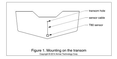
Mount the sensor near the centerline and close to the bottom of the transom.
