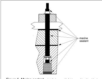
Figure 5. Marine sealant—detail shown with fairing and backing block Copyright © 2000 - 2018 Airmar Technology Corp.
