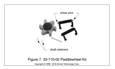
Replace broken or worn parts immediately. The water-lubricated paddlewheel bearings have a life of up to 5 years on low-speed boats [less than 10kn (11MPH)] and 2 years on high-speed vessels.
