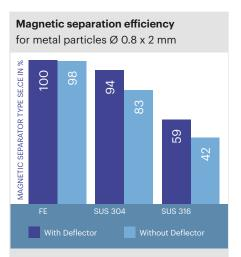
The effectiveness graph shows what you can expect from an Easy Cleanflow magnet. The idea is to allow you to enter product parameters so you can know for certain which particles will be captured. We utilize a computer simulation process in which we can change the parameters to match various products. These could be anything from milk powder to cocoa powder or even quartz sand. This enables us to make a prior assessment of the expected effectiveness of our magnetic separators.
