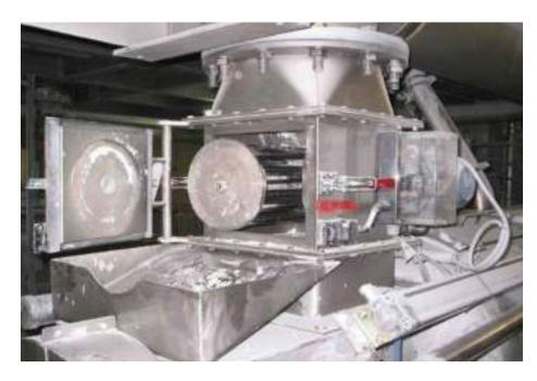
advantages: the magnetic field strength at the pipe is considerably higher. This is important for capturing 316 stainless steel particles. Moreover, no product comes between the magnetic bar and the extractor tube.
