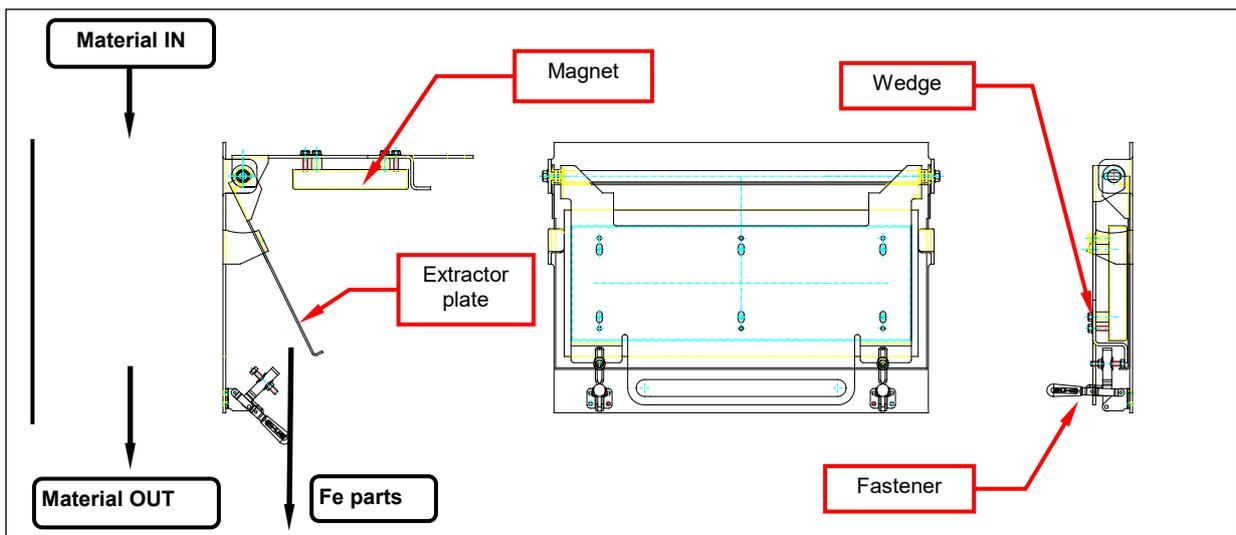
**Drawing:** Plate magnet – type quick-cleaning (with extractor plate)
