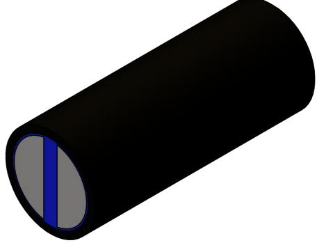
DIRECT MOUNTING OF THE BAR MAGNET IN IRON REDUCED THE HOLDING POWER BY UP TO 15% DUE TO MAGNETIC SHORT CIRCUITING. TO AVOID THIS CERTAIN DISTANCES NEED TO BE MAINTAINED BETWEEN THE BRASS CASING OF THE BAR MAGNET AND THE IRON. THE DISTANCE ARE ALSO TO BE ADHERED TO IF THE BAR MAGNET WAS SHORTENED BY DIMENSION A. PLEASE REFER TO THE DISTANCE GIVEN IN THE DRAWING (distance .... mm).
