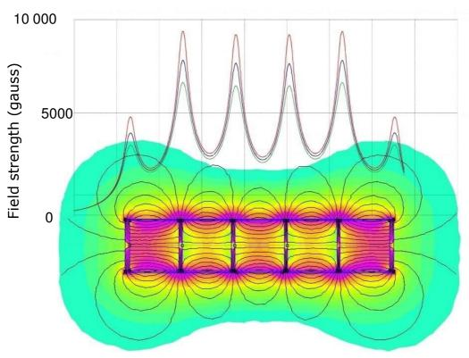
Magnetic bar Ø23 mm (GSN-42) in extractor tube Ø25 mm
