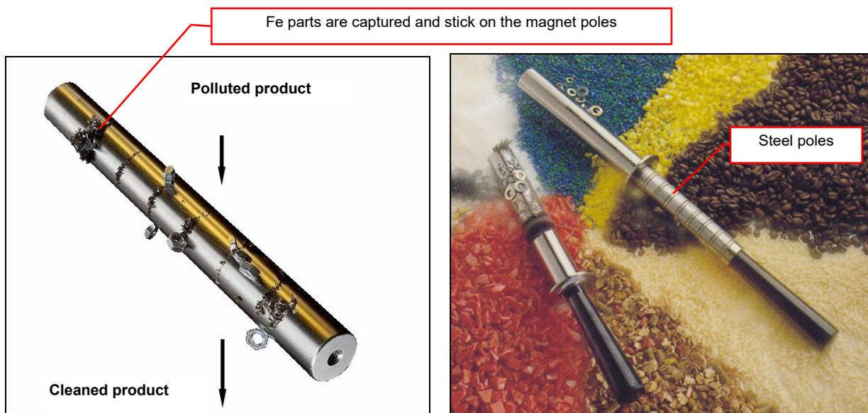
**Photo:** magnetic bar with surrounding SS tube
