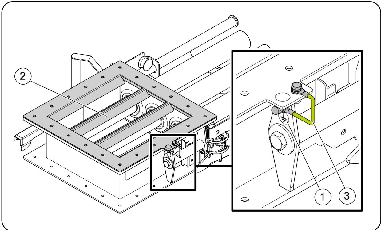
A deflector [2] is optionally available to ensure that all particles of the product stream touch the bars. The deflector is standard equipped with a earth wire [3].
