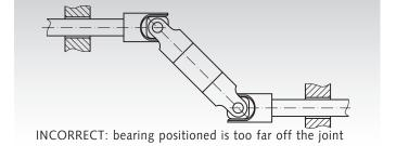
The universal joints are supplied without pinholes and split pins. The length of the split pin is determined by the outer diameter of the universal joint, i.e. the pin must be flush when inserted.
