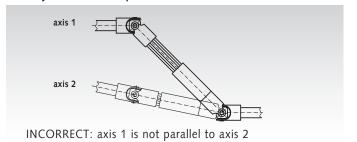
4. The universal-joint shaft - or the double universal joint - should be supported as close as possible to the universal joints.
