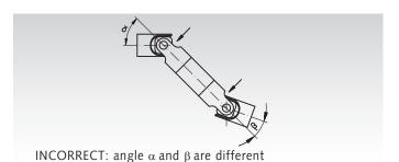
3. When position of driving and driven shaft is changed, they must always be moved in parallel.
