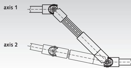
INCORRECT: axis 1 is not parallel to axis 2
