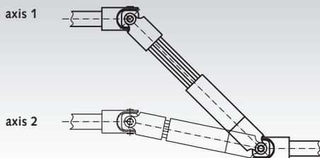
CORRECT : axis 1 is parallel to axis 2
