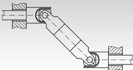
CORRECT : bearing positioned as close as possible
