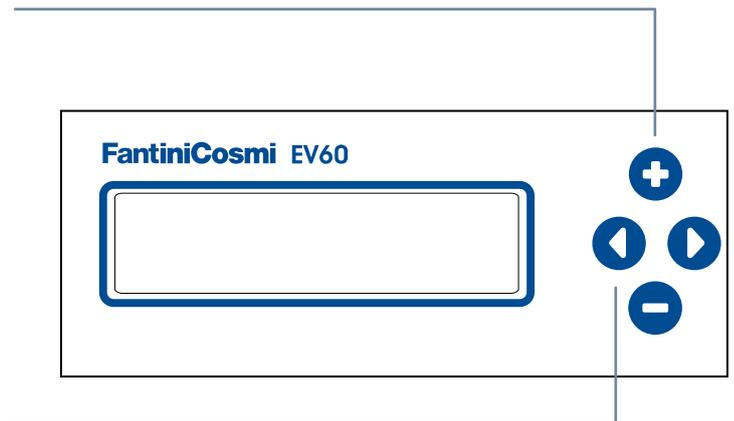
EV60 control unit continuously compares the measured temperature with the one preset (which depends of the current programming). Based on the proportional band and the integral time, it determines the position of the regulating mixing valve or commands the two stages of the output relays.
