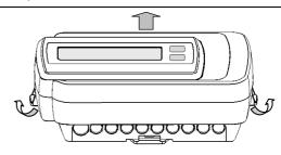
Open the calculator by acting on the two side hooks to remove the upper assembly with the electronic section.
