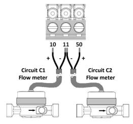
The connection example refers to a system fitted with four pipes, with separate heating and cooling circuits.
