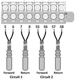
The example refers to a system fitted with four pipes, with separate heating (Circuit 1) and cooling (Circuit 2) circuits.
