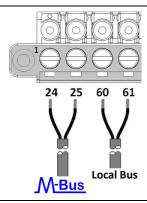
Polarity needs not be complied with for both connections; however, it may be recommended that you should keep the same polarity for the entire wiring, due to system-related reasons.
