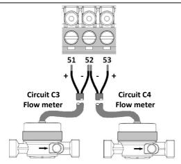
The connection example refers to the use of both pulse inputs. If one or both inputs are not used, their respective terminals shall be left open (not connected).
