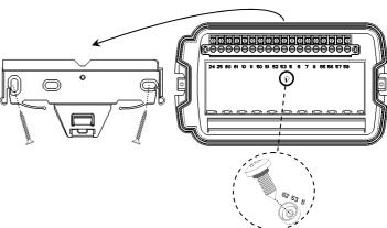
Remove the fastening bracket from the bottom section and fix it to the wall; then, fit the bottom onto the bracket and fix it by making use of the "anti-removal" kit (i.e. screw and O-ring) supplied together with the unit.
