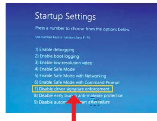
After rebooting the system, you can continue the installation of the driver of the USB Optical Head, referring to the procedure for installing the driver for Windows 7/Vista (pag.7).
