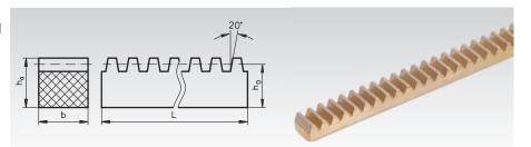
Ordering Details: e.g.: Product No. 260 601 00, Straight-Toothed Gear Rack, Module 0.3, 250 mm The teeth on the gear racks are manufactured using an overhead milling cutter. This leads to negative tolerances. Dimension  $h_a$  and  $h_0$  up to module 2 -0.2 mm.
