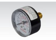
**Materials:** Housing, viewing glass: Plastic. Connecting thread: Brass. Operating pressure: 0-10 bar.  $T = -20^{\circ}C$  to  $60^{\circ}C$
