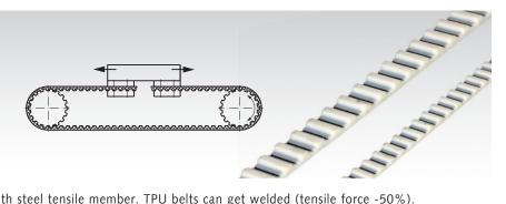
Material: Thermoplastic polyurethane (TPU), with steel tensile member. TPU belts can get welded (tensile force -50%). Ordering Details: e.g.: 160 600 00, Open-Length Timing Belt T 2.5, Width 6 mm.
