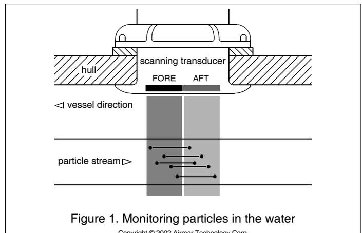
Figure 1. Monitoring particles in the water
