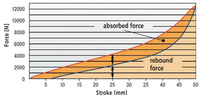
With aid of the characteristics curves above you can determine the amount of energy that will be absorbed.
