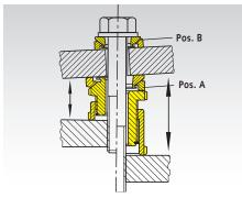
Like the ball head precision adjusters MN 686.4 the ball shim MN 686.5 (Pos. A) facilitates adjustment of non-parallel surfaces with an angle of inclination of up to 4°. If the angle of inclination  $\alpha > 1$ °, the use of an additional ball shim (Pos. B) is recommended to assure a stable support of the bolt head.
