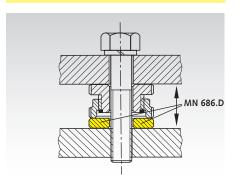
The Spacer MN 686.D is used to bridge gaps between the levelling adjuster and the bearing surface when the adjustment travel  $\Delta h$  is insufficient.
